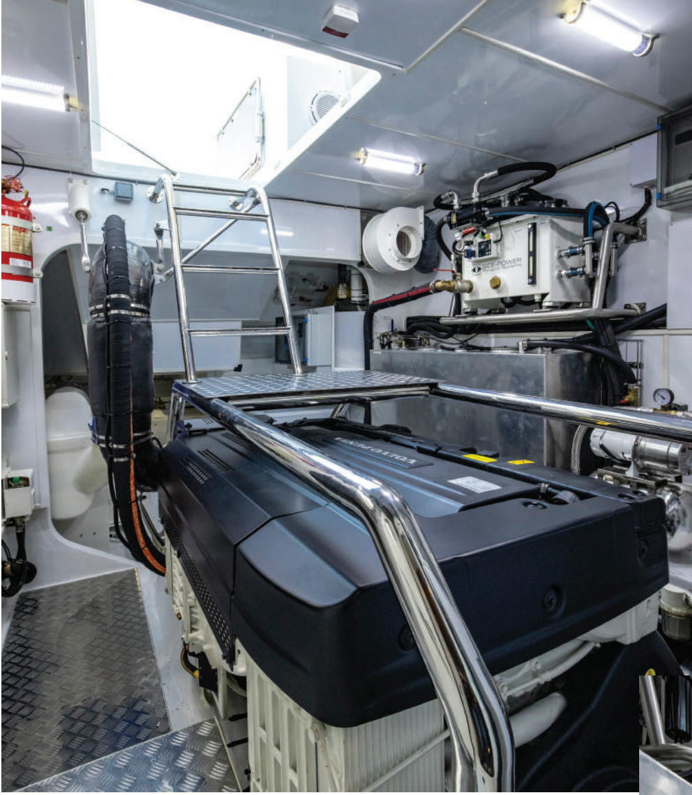
2X D13 1000 HP Volvo Penta Diesel Engines.
